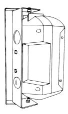
bracket. When used vertically as shown attached to a wall, the enclosure is free to rotate in the horizontal plane over more than 180°. It can also be turned through 90° and mounted horizontally on to a wall in which case the enclosure can be tilted downwards to give the desired coverage. The SB-50 can also be fixed to a ceiling, again allowing for a wide range of adjustment of the enclosure.
